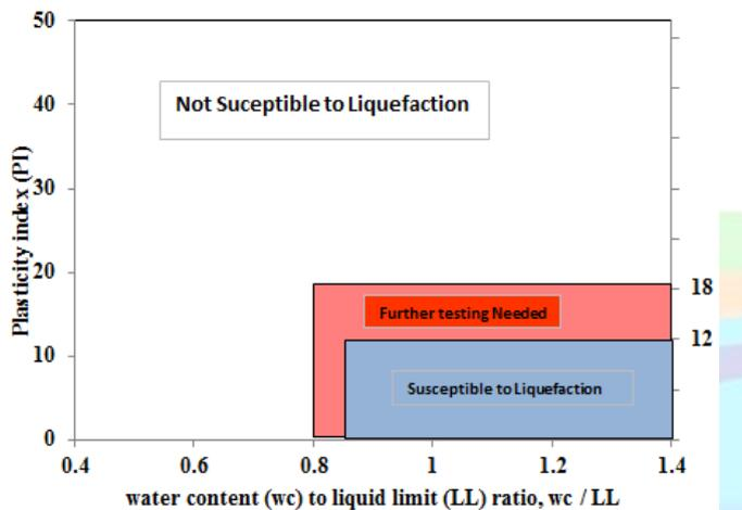
Fig.3: Liquefaction susceptibility margins proposed by Bray and Sancio (2006)
