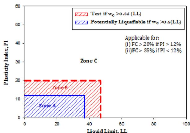
Fig.2: Recommended liquefaction susceptibility boundaries for fine-grained soils by Seed et al. (2003)
