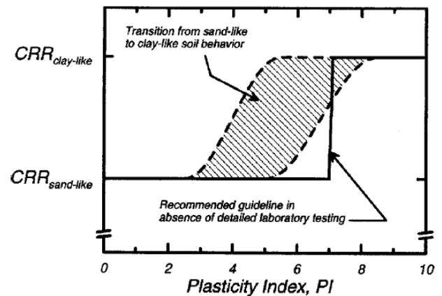
Fig.4: Schematic Illustration of the transition from sand-like to clay-like behavior for fine-grained soils with increasing  $PI$ , and recommended guideline for practice. (After Boulanger & Idriss, 2006)
