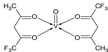
Figure 6: Suggested structure for Oxovanadium Bis(trifluoroacetylacetonate) chelate complex.
